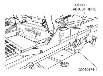
Figure 6-6. Cutter Deck Level Adjustment
